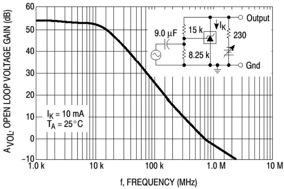
**Figure 12. Open-Loop Voltage Gain versus Frequency**
