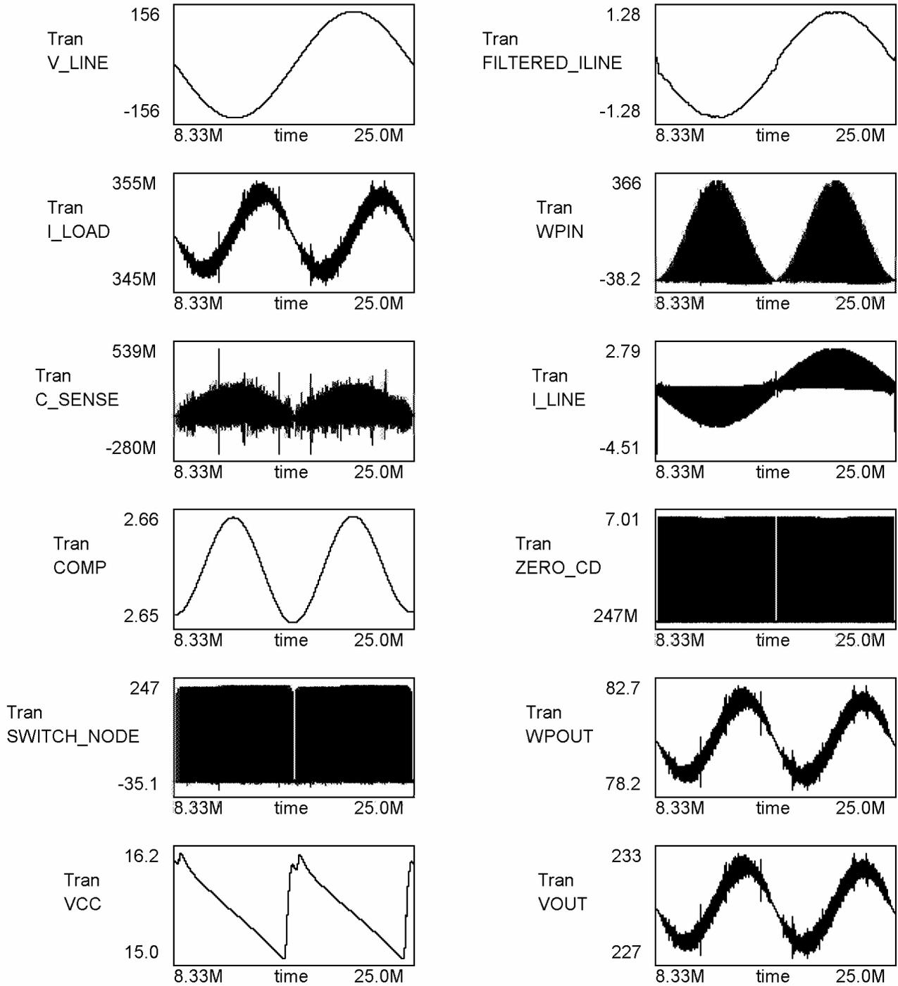
**Figure 5.4.7: Spice Application Output Waveforms**
