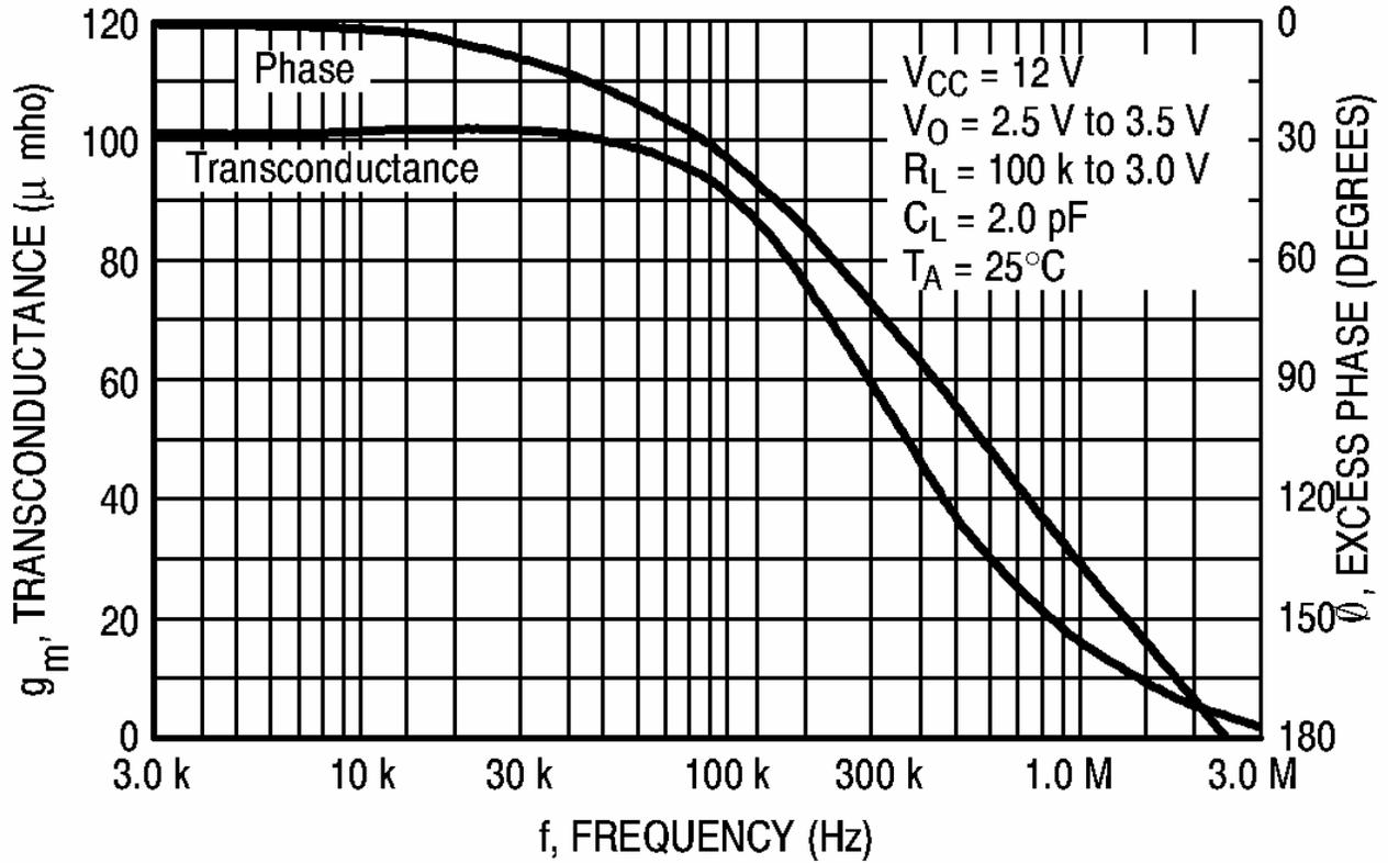
**Figure 5.4.4. Error Amp Transconductance & Phase of Actual Data plots**
