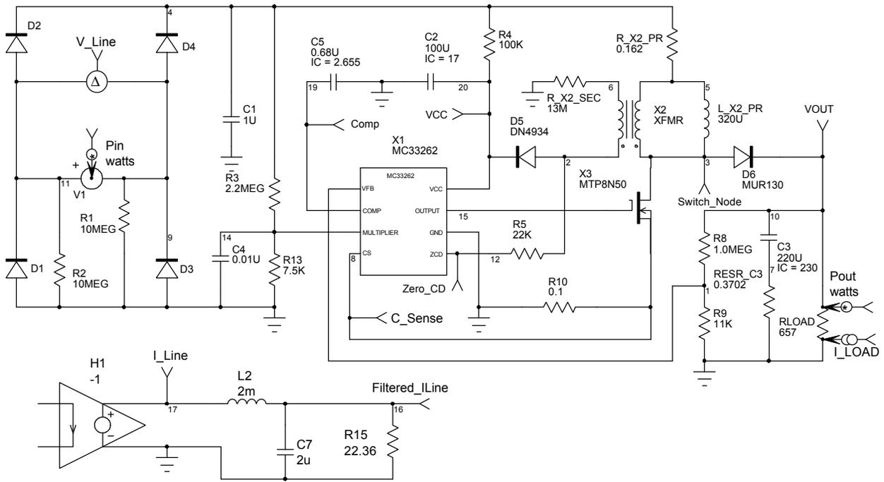
**Figure 5.4.5: 230V/0.35A Power Factor Spice Application Diagram.**
