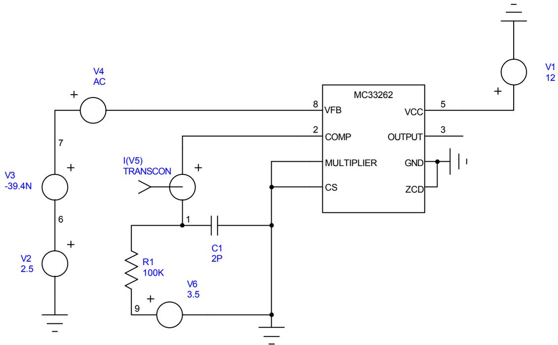
**Figure 5.4.1. Error Amp Transconductance and Phase Test Fixture.**
