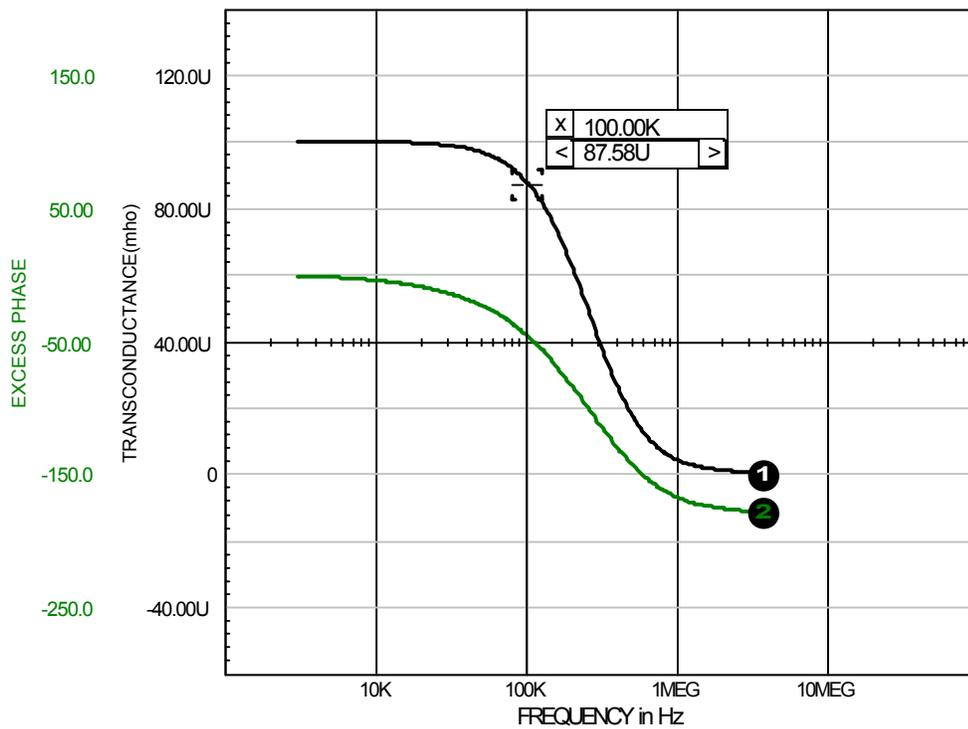
**Figure 5.4.3. Error Amp Transconductance & Phase versus frequency plots**
