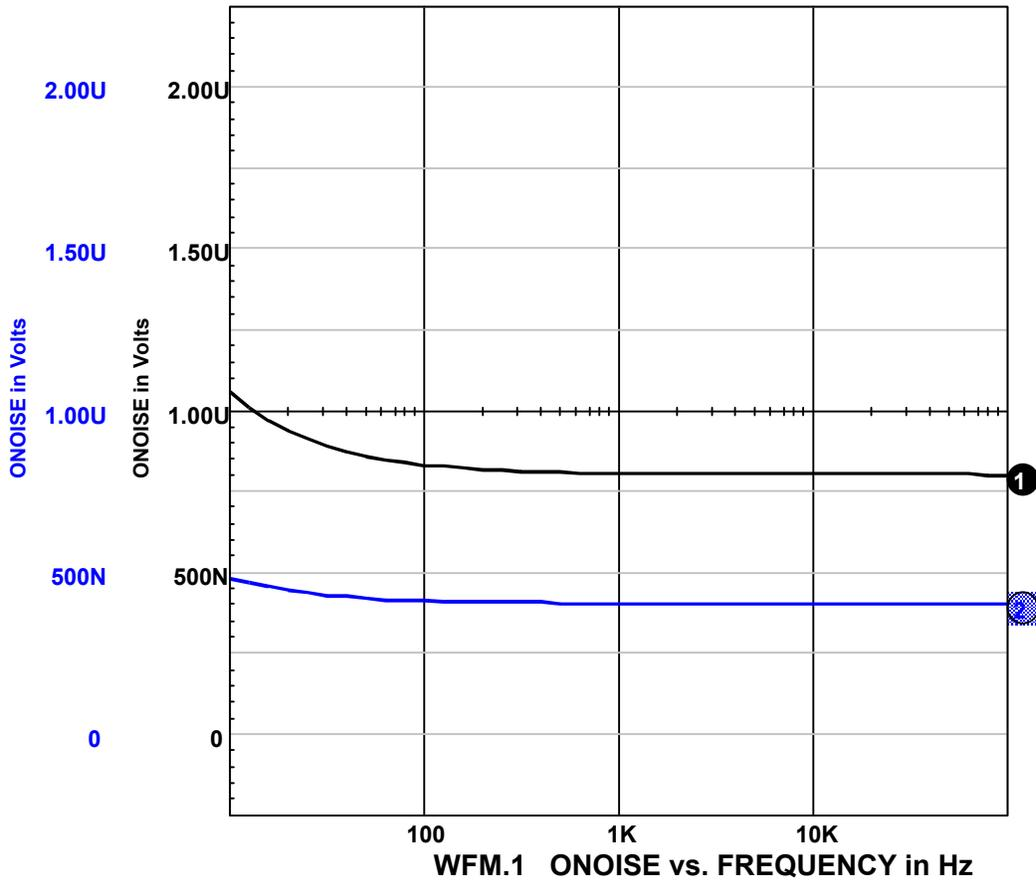
**SPICE Waveforms Noise spectral density (RTO)**
