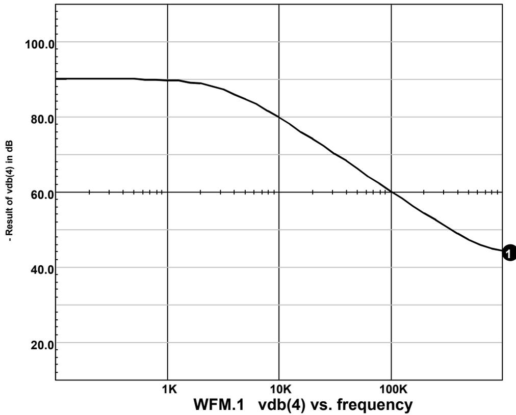
SPICE Waveform of common mode rejection
