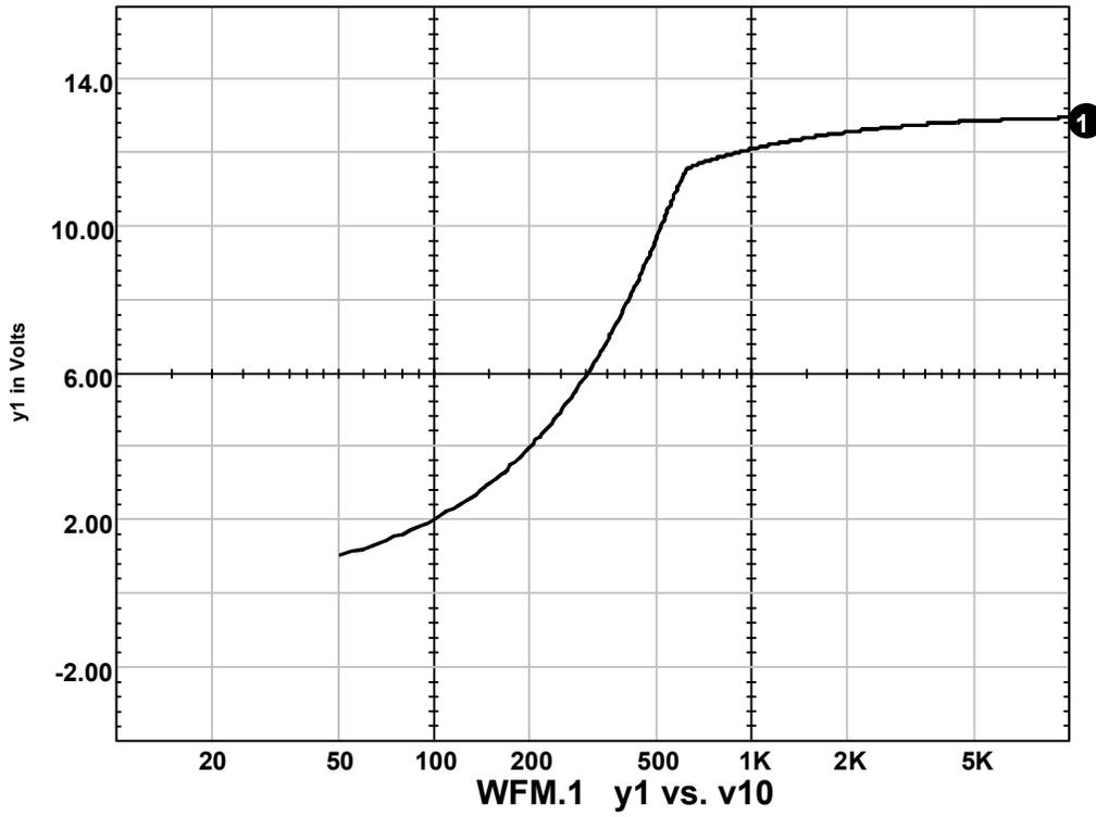
**SPICE Waveform of output voltage swing vs. load resistance**
