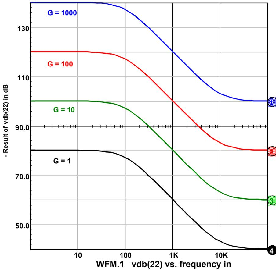
**SPICE Waveform of common mode rejection**
